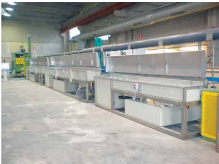
High speed zinc plating
