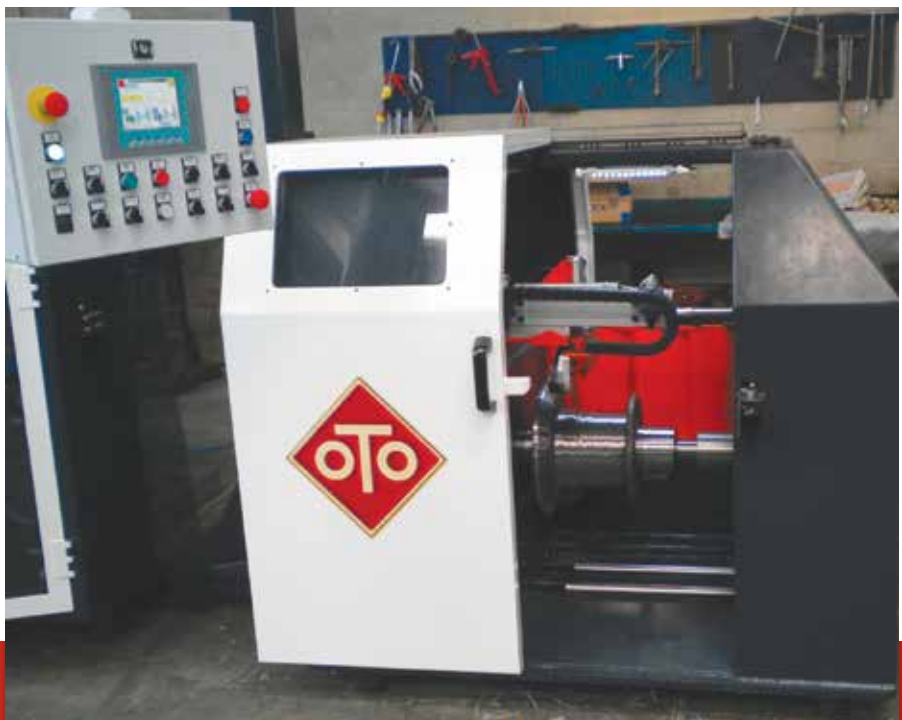
Automatic change over of baskets and spool
