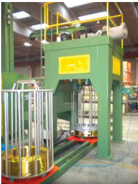
Automatic change over of baskets and spool
